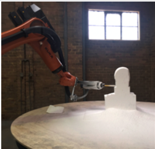
Figure 72. Robotic milling and drilling system
