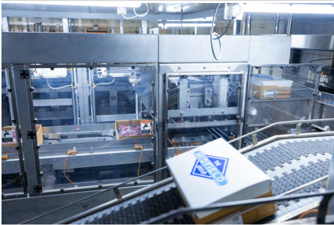
Figure 56. MHM's carton lifter
